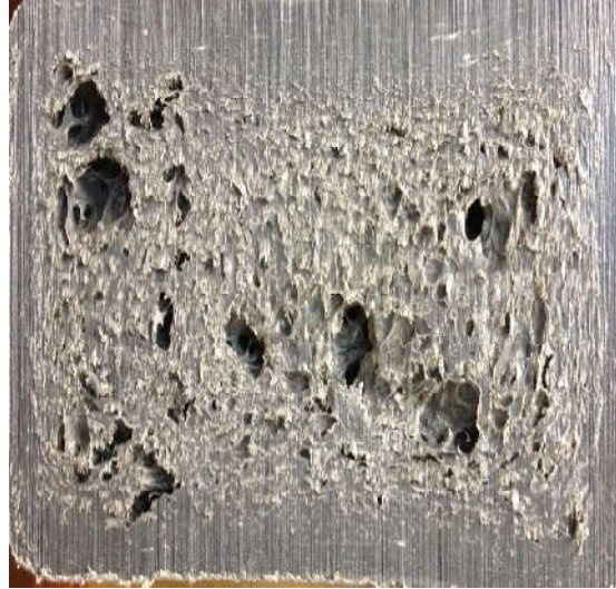
Figure 3 Presence of voids in the core region with stiff borders.
