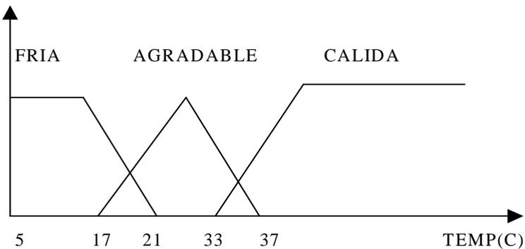
$\text{TEMP}(18) = \{0.5/\text{FRIA}, 0.2/\text{AGRADABLE}, 0/\text{CALIENTE}\}$
