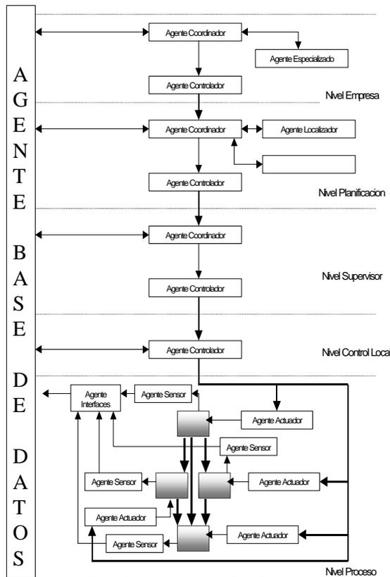
**Figure 4.** The tank control model using IDCSA
